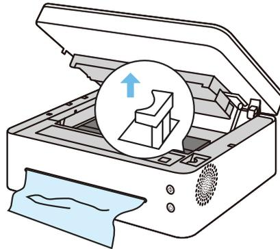
**4** Pull the jammed paper carefully out of the paper exit.
