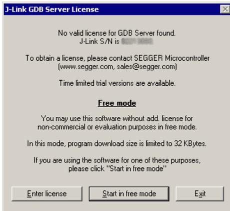
Select **Start in free mode** to start J-Link GDB Server with 32 Kbytes download limitation or select **Enter license** to remove the limitation and deactivate the startup dialog. If the J-Link GDB Server is started in free mode, a status message appears in the log window.
