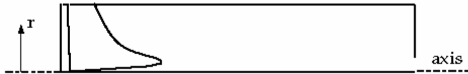
Figure 1: Typical Radial Distribution of w in a Free Vortex
